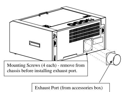
As part of the unpacking process you will find a 4" (100mm) exhaust port in the accessories kit. This part needs to be attached to the rear of the Mini chassis before connecting the Exhaust blower to the Mini.
