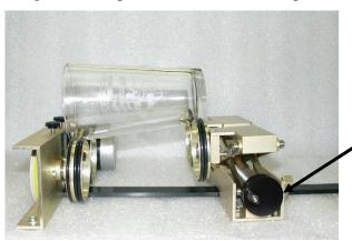
Use the elevator on the rotary attachment to raise the right side of the object being engraved so that its engraving surface is horizontal.
