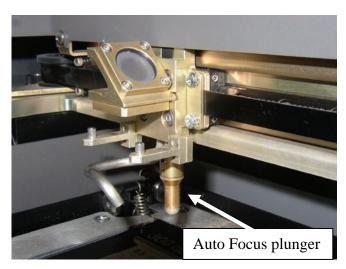
Checking the box will activate the Auto Focus process when the job starts to run.
