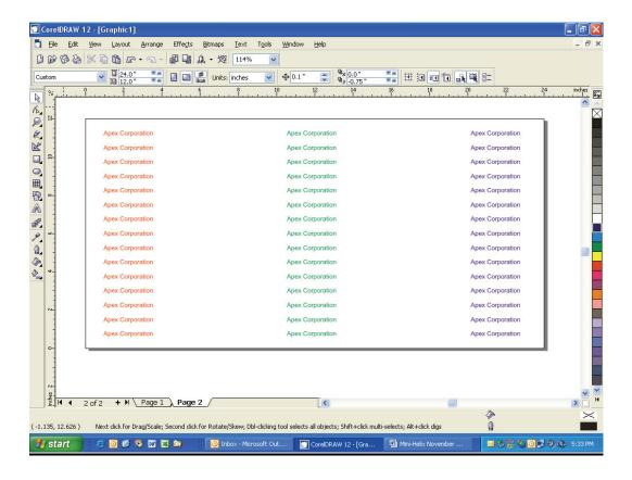
For the above example we've assigned all of the names in the first column the color red, the second column the color green, and the third column, blue. In the Dashboard you will follow the same process that was used in Vector Color Mapping for setting up the Raster Color Mapping colors, but for this example we will assign all colors the same speed and power (see following diagram).
