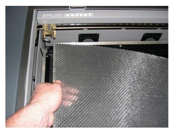
On the Mini 24 x 12 and the Helix there is an insert that supports the Vector Grid. This insert is held in place by notches in the table and it simply lifts out.
