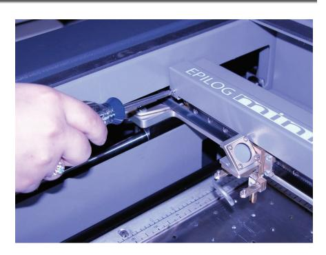
The X-beam with the cover removed. This photo shows the air assist tube and support.
