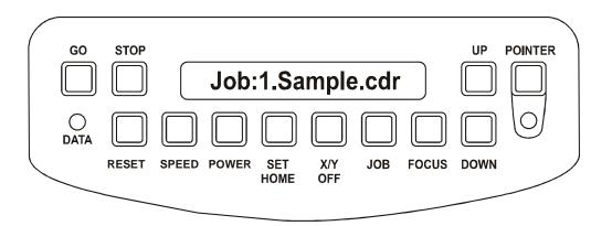
Once the job starts, the display changes to show a job timer and the engraving resolution. The timer is a useful production tool that displays the elapsed time of engraving.
