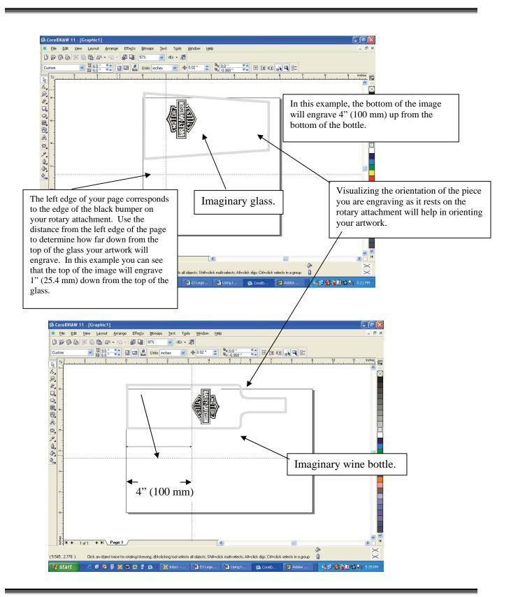
If placement of your artwork is critical, many users place a couple layers of masking tape onto the area of the glass to be engraved and practice at high speed and low power to mark only the tape.
