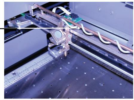
The optical strip is a thin, clear piece of plastic that has very thin, small vertical lines on it. The strip runs the length of the x-beam from left to right. The cotton swab is shown on the front side of the strip.
