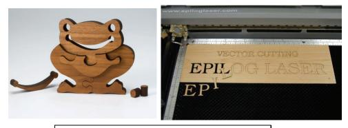
The two samples above show the results of Vector Cutting in wood.
