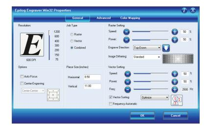
Now that you have printed a simple job, you are ready to gain a better understanding of the different printing options available from the Dashboard. Most engraving and cutting jobs can be accomplished by using only the General tab. Advanced features for more complex jobs can be found under the Advanced and Color Mapping tabs.
