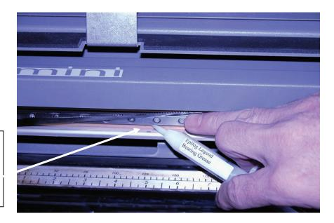
This photo shows the location of the X-axis carriage and the X-axis bearing (which is behind the X-axis belt.
