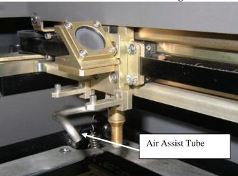
stream helps reduce charring and scorching associated with materials, such as wood, rubber, and acrylic.
