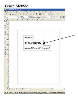
The Fence method uses a *closed* outline to define the area to be engraved away. This image shows the stair-step outline of a Fence enclosing the words to be stamped. The laser will engrave away only the background area outlined by the Fence (leaving the letters standing, of course!).
