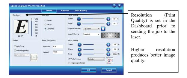
Speed and Power settings are dependent on resolution setting. For example, there is greater overlap of each raster line at 600 DPI than there is at 300 DPI. The additional overlap at 600 DPI has the effect of lasering over more of each line twice. This means that on material like wood, you will notice a greater depth of engraving at 600 DPI than you will at 300 DPI if you use the same Speed and Power settings.
