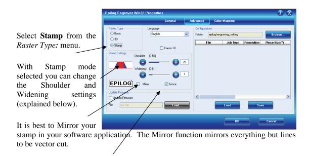
Check the Fence box if necessary.
