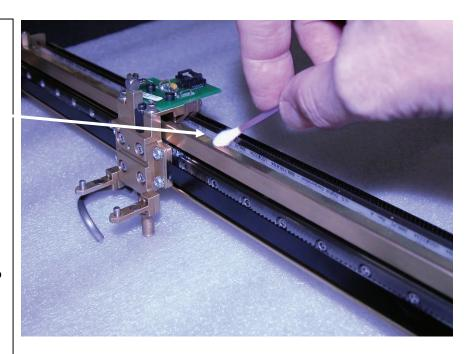
This photo shows the encoder. The encoder is a horseshoe shaped device that straddles the encoder strip. There is a slim possibility that dirt and debris can get up inside the encoder. Blow some compressed air under the encoder to remove any dust and debris.
