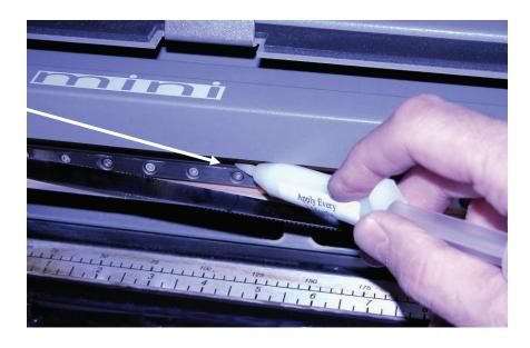
Place a bead of grease along the bottom groove of the X-axis rail.
