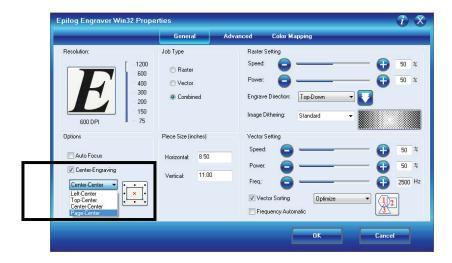
The Center Engraving Option allows you to define the center of your artwork as the primary reference point (Home position) of your engraving or cutting. The Center Engraving Option has been designed to be used in conjunction with the Set Home feature of the laser. This differs from standard printing where the upper left corner of the page and the upper left corner of the laser table define your primary reference point. There are four options for centering your artwork:
