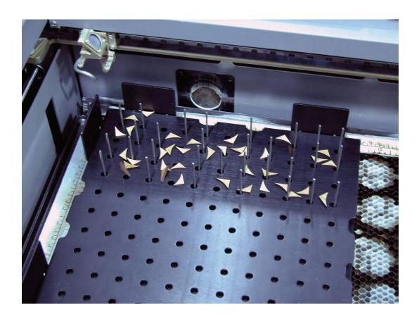
The following photo shows two Pin Tables lined up side by side. You can use as many Pin Tables as your table will allow.
