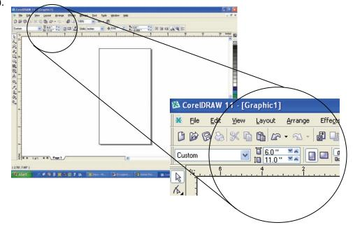
Place your artwork close to the top edge of the page layout. When the job starts the engraving process, the first thing to happen is for the rotary attachment to rotate through any white space that is between the top of your page and the top of your artwork. Once it has rotated through the white space it will begin to laser your artwork.
