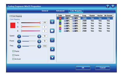
Make sure Color Mapping is checked so we can set up our color mapping scheme.
