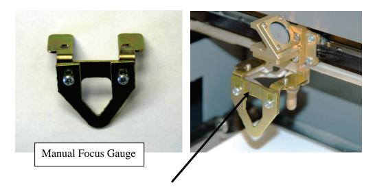
Place the manual focus gauge on the carriage. Use the *Focus* button and the *Arrow Keys* on the front control panel to move the table up until your material just touches the bottom of the gauge. Once the focus position has been established, remove the gauge. Press the *Reset* button to return the carriage to its "Park" position before starting your job.
