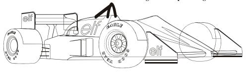
The upper image is a complex piece of clipart. The lower image shows all of the hidden lines that are in this piece of clipart. If this clipart image were run in *Combined mode* it would first raster most of the car then vector cut all but the thickest lines.
