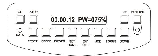
Pressing the **POWER** button while raster engraving will change the display to show the Power setting of the job while it is running (see diagram above). Pressing the **UP** or the **DOWN** key will increase or decrease the power output of the laser in Raster Mode. Normally you will need to increase or decrease the Power by 10% or more before you start to notice a visible change. You cannot change Power on the fly in Vector mode.
