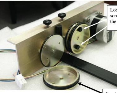
Loosen the two small thumb screws on each wheel to remove the front wheel.
