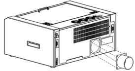
the laser system to the intake side of the exhaust fan. Then connect the exhaust side of the exhaust fan to the metal duct leading outside.
