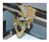
left corner of the machine. Press **Focus** on the keypad, then use the Up and Down Arrows to move the table to the correct height. Once the focus position has been established, remove the gauge. Press the **Reset** key.
