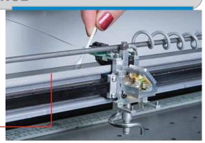
The encoder reader is a horseshoe shaped device that straddles the encoder strip. There is a possibility that dirt and debris can get inside the encoder. Blow some compressed air under the encoder to remove any dust and debris.
