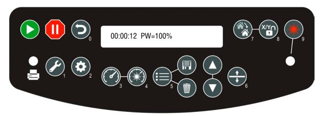
Pressing the power key while engraving will change the display to show the power setting of the job while it is running. Pressing the Up or Down arrow key will increase or decrease the power output of the laser in raster mode. Normally you will need to increase or decrease the power by 10% or more to see a visible change in the laser's speed.
