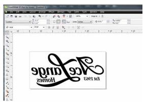
**Creating a Perforated Cut:** To create a perforated cut around the stamp that will allow the stamp to be pulled away from the rubber, in the print driver set the vector frequency below 100. This keeps the stamp attached to the rubber sheet and makes cleaning easy while allowing the user to easily remove the stamp from the sheet.
