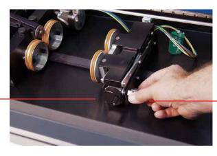
Flip the release lever to move the scissor jack left and right.
