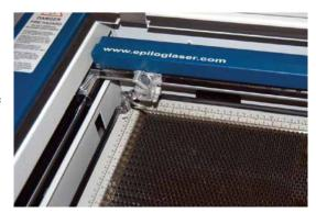
There is a leveling bar located below the vector cutting table that should always be in place to have the most level cutting table possible. To access the bar lift the rulers and remove the gridded table.
