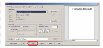
At this point, the .hex file will begin transferring to your laser. The laser knows that it is being upgraded and the graphic that you created will not print, nor will it show up as a Job. Instead, the cursor keys will light up. When the upgrade is complete, the display will read **Reboot!**
