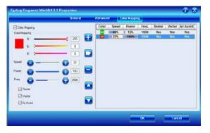
7. In our example we want to mark the green window frames first, so green must be the first color at the top of the list. Normally the color green is the second color down in the list. In order to move it we just select it and press the **Up key** to move it up one position. We now have green at the top and red is the second color down. This is the order in which the colors will be processed.
