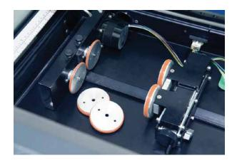
There are two small thumbscrews that attach each front drive wheel to the back drive wheel. Loosen the two small thumbscrews on each wheel to remove the front wheel.
