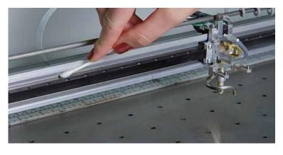
the bottom side of the rail. You will need to move the X-axis belt out of the way to access the rail. There is enough flex in the belt to move it out of the way, but do not pull on it so hard that it becomes stretched or stressed.
