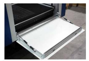
The front access door is usually used for easy loading and unloading of palletized materials. The door is interlocked and the laser will not fire if the door is open.
