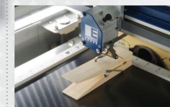
2) Measure the clothespin to locate the center and mark and lightly mark an x with a pencil. Place the clothespin in the system and set the focus. Utilize the Red Dot Pointer to locate the marked center, set your home position and press Go!
