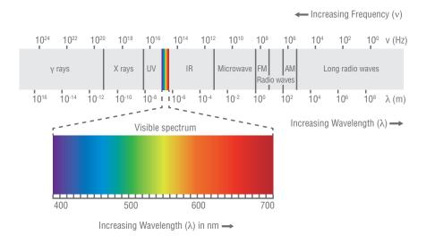
For purposes of understanding lasers, we generally think of light as electromagnetic radiation having wavelengths ranging from around 10 nm (the bottom of the ultraviolet, or UV, portion of the spectrum) up to about 1,000,000 nm (or 1 mm, the top of the infrared, or IR portion).
