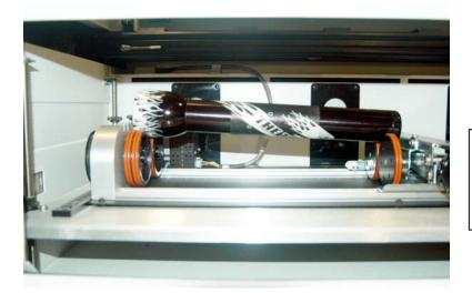
**Incorrect Setup** – The flashlight is not horizontal. Raise the right side of the flashlight by turning the jack screw.
