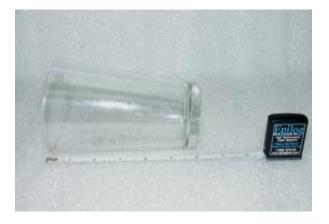
For the width (x-direction) of your page, lay the glass flat and orient it as it will be oriented on the rotary attachment. For this glass, the width of the page will be six inches (152 mm).
