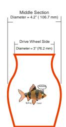
Divide the drive wheel side by the middle diameter and multiply by 100 to calculate the percentage of adjustment. For our example the calculation is:
