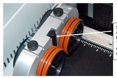
Set your cylinder on the rotary attachment so that it is close to the black bumper, but not touching it. The cylinder may not be able to rotate freely if it is rubbing against the bumper. The "top" of a cylinder can be at either end of the rotary attachment. It is useful to visualize the orientation of the cylinder when it's being engraved.
