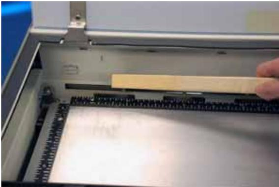
Clean the vents from the inside of the machine. It is best to use a flexible plastic or wire brush that can access the inside of the vent.
