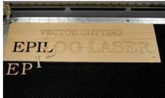
The two samples above show the results of Vector Cutting in wood.
