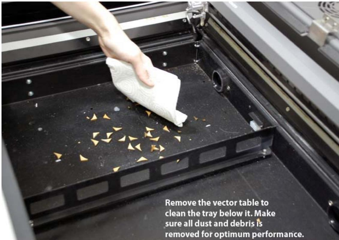
**Remove the vector table to clean the tray below it. Make sure all dust and debris is removed for optimum performance.**
