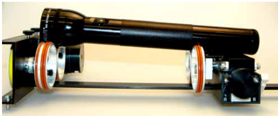
Incorrect Setup. Flashlight is not level.
