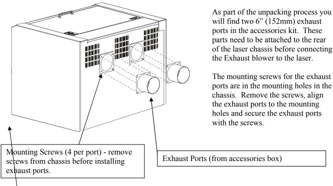
will find two 6" (152mm) exhaust ports in the accessories kit. These parts need to be attached to the rear of the laser chassis before connecting the Exhaust blower to the laser.
