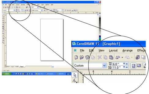
Place your artwork close to the top edge of the page layout. When the job starts the engraving process, the first thing to happen is for the rotary attachment to rotate through any white space that is between the top of your page and the top of your artwork. Once it has rotated through the white space it will begin to laser your artwork.
