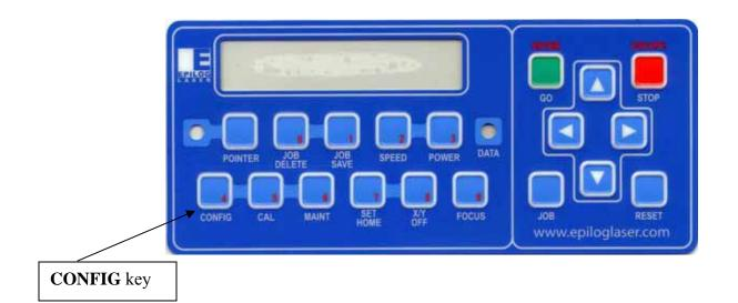
To access these settings, press the **CONFIG** key. After pressing the **CONFIG** key, use the Up or Down cursor keys to scroll to the desired field.
