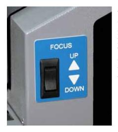
There is one last method of focusing. When the large front door is open and you want to manually focus it is hard to do because the keypad is out of reach on the top of the door. There is a switch at the left front of the engraving cavity that allows you to move the table up and down to manually focus with the door open.
