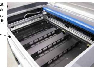
Once the task plate or vector grid is removed, and supports are also removed, you will see the three mating holes in the bottom of the table tray. These holes mate to the pins in the bottom of the rotary attachment.
