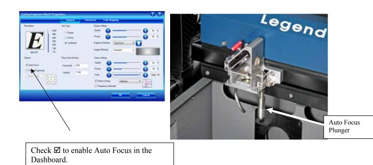
When the *Go* button is pressed and a job is started, the carriage will move from the upper left corner to the first point of engraving. Once it reaches the first point of engraving the table will move up if Auto Focus was activated when the job was printed. It is important that there are no obstructions in the path of the carriage between the upper left corner and the first point of engraving.
