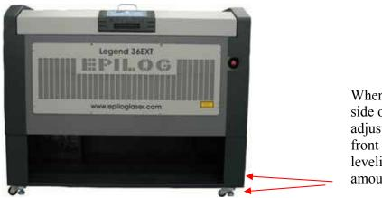
When raising the right side of the machine adjust both the right front and right rear leveling feet the same amount.
