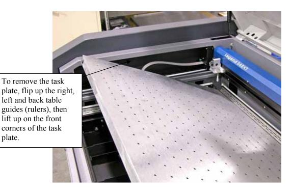
The task plate is a very rigid one inch thick removable perforated work surface. It is normally used in engraving mode and it has several interesting features:
