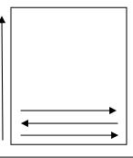
Bottom-Up engraving starts from the bottom and works its way up.
