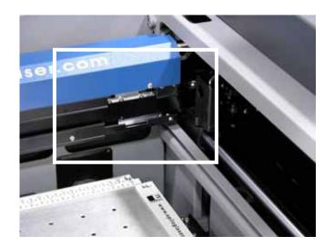
The beam splitter/lens assembly has a locating hook on the bottom of the assembly and two Phillips head screws that secure it to the secondary bearing block. The assembly is designed so that the x-belt travels freely between the bearing block and the beam splitter/lens assembly.
