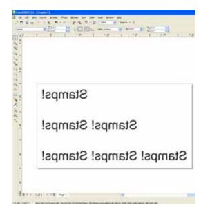
The Fence method uses a *closed outline* to define the area to be engraved away. This image shows the stair-step outline of a Fence enclosing the words to be stamped. The laser will engrave away only the background area outlined by the Fence (leaving the letters standing, of course!).
