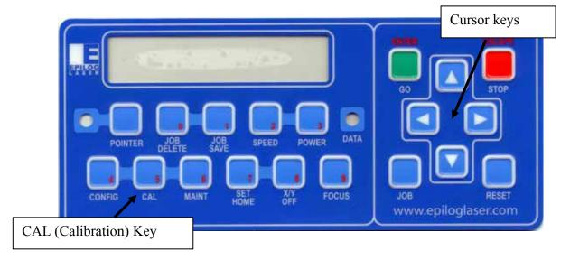
To access additional fields press the Down cursor key. Once the field is displayed its value can be adjusted by pressing either the right or left cursor keys. Pressing the **GO/ENTER** key saves the change. Pressing the **STOP/ESCAPE** key exits the Calibration menu without saving changes.
