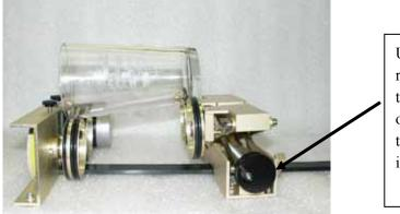
Use the elevator on the rotary attachment to raise the right side of the object being engraved so that its engraving surface is horizontal.
