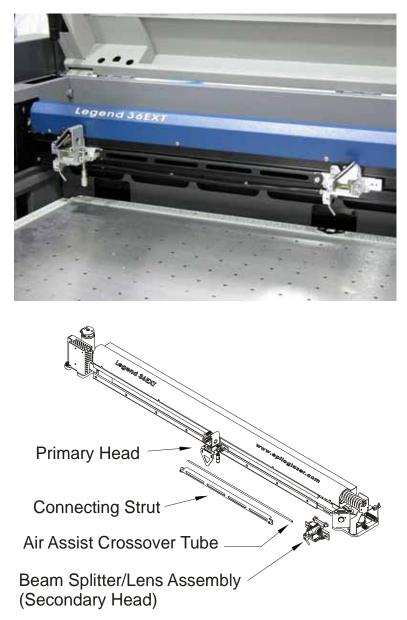
When you are finished using the Double Head, turn the machine off, disconnect the strut, and the air assist crossover tube then remove the beam splitter/lens assembly. "Park" the bearing block at the far right side of the bearing rail.
