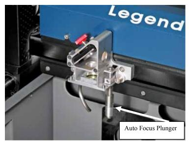
When a job is started and Auto Focus has been enabled the carriage will move from its park position to the point of first engraving or cutting. Once it finds this first point the table will automatically move up and push the plunger up. Because the carriage moves to the start point before focusing it is necessary to have enough clearance between the bottom of the Auto Focus plunger and the top of the
