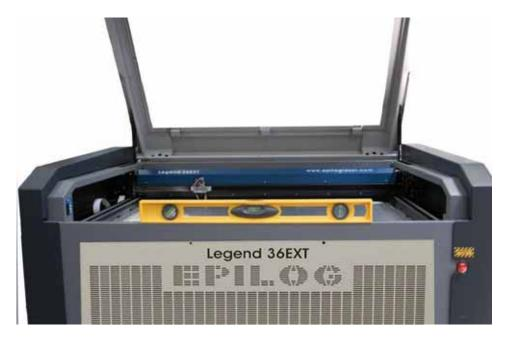
6. Locate the level's center indicator. The center indicator bubble shows the level of the machine.
