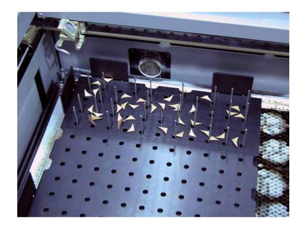
The following photo shows two Pin Tables lined up side by side. You can use as many Pin Tables as your table will allow.
