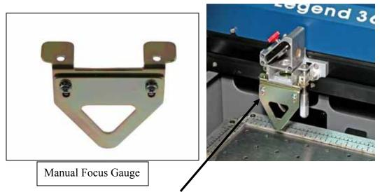
Place the manual focus gauge on the carriage. Use the *Focus* button and the *Arrow Keys* on the front control panel or the *Focus Key* inside of the laser cabinet to move the table up until your material just touches the bottom of the gauge. Once the focus position has been established, remove the gauge. Press the *Reset* button to return the carriage to its "Park" position before starting your job.
