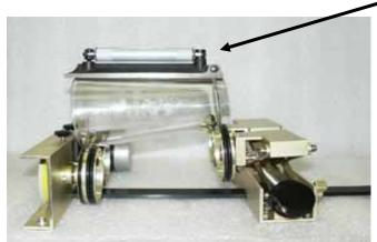
The photo below shows a typical setup for something other than a glass. The larger diameter is on the left side of the rotary attachment and the right side of the flashlight has been elevated so that it is resting horizontally.
