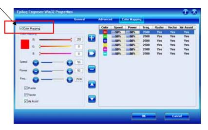
The Color Mapping feature is an advanced feature that must be checked to activate. While Color mapping is a very powerful tool, most users use it for two main reasons:
