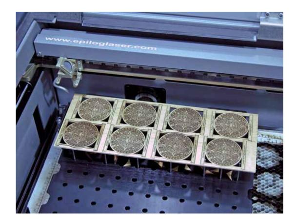
The photo below shows the small pieces from the previous photo laying on the Parts Lifter. Simply lift the Parts Lifter from the Pin Table and throw away the pieces. Cleaning up with the Parts Lifter makes clean up easy because you do not have to remove the Pin Table from the machine, nor do you have to pick up each individual waste piece from the machine. Simply clean off all of the waste pieces and replace the Parts Lifter onto the Pin Table.
