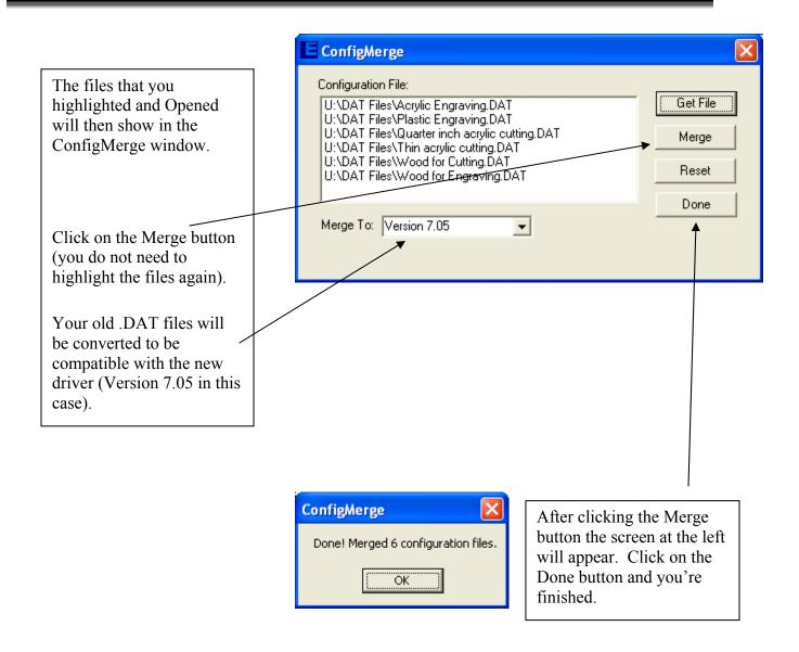
The Merge feature does not delete the old .DAT files. It creates new files using the same name, but adding the new driver version number (\_705 in this case). In the following screen you can see that the original file is named Acrylic Engraving.DAT. The merged file is named Acrylic Engraving\_705.DAT.
