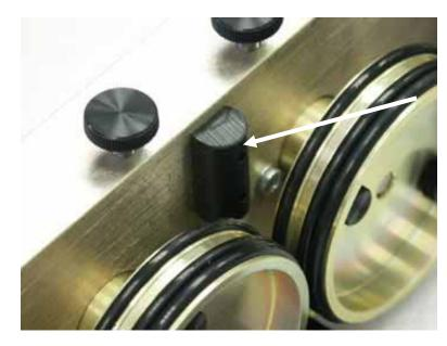
Set your glass on the rotary attachment so that it is close to this bumper, but not touching it. The glass may not be able to rotate freely if it is rubbing against the bumper
