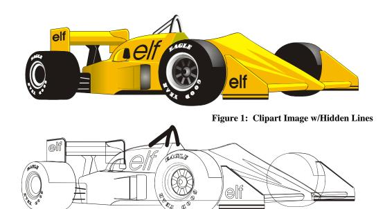
The upper image is a complex piece of clipart. The lower image shows all of the hidden lines that are in this piece of clipart. If this clipart image were run in *Combined mode* it would first raster most of the car then vector cut all but the thickest lines.
