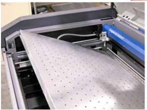
On the EXT there are four inserts that support the Vector Grid and Task Plate. The inserts are held in place by notches in the table and they simply lift out.
