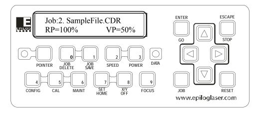
Pressing the **POWER** button while raster engraving will change the display to show the Power setting of the job while it is running (see diagram above). Pressing the  $\hat{U}$  **UP** or the  $\frac{1}{2}$  **DOWN** cursor key will increase or decrease the power output of the laser in Raster Mode. Normally you will need to increase or decrease the Power by 10% or more before you start to notice a visible change. You cannot change Power on the fly in Vector mode.
