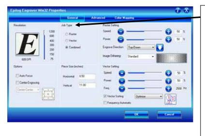
The Job Type: menu allows you to specify Raster, Vector, or Combined. This setting works in conjunction with the way your artwork is setup to produce a raster engraving, a vector profile, or a combination of the two modes in a single job.
