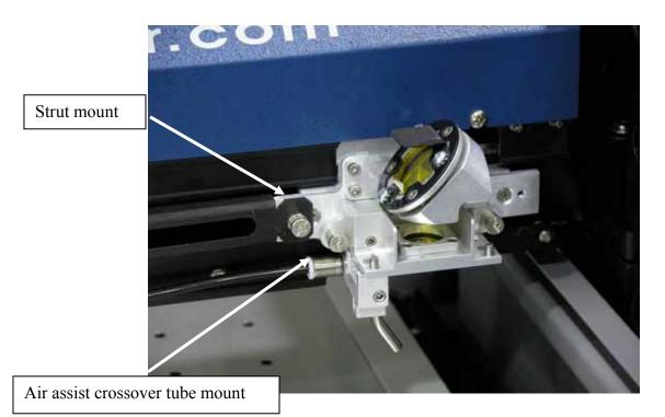
Attach the strut and the air assist crossover tube to the primary head and the installation is complete.
