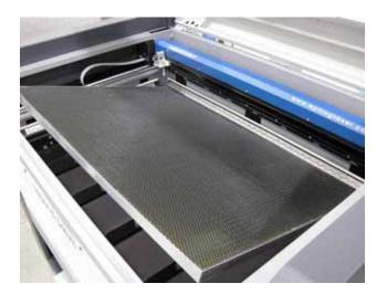
Honeycomb Vector Grid being installed into a 36 EXT.
