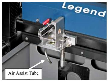
assist removes the heat and combustible gases from the work surface. The constant air stream helps reduce charring and scorching associated with materials, such as wood, rubber, and acrylic.
