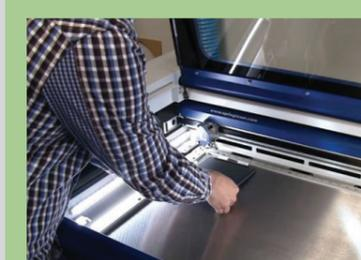
**Tip:** For best results, select the "Bottom-Up" engraving option and Stucki dithering pattern. Engraving from the bottom up helps ensure any engraving debris/residue is pulled up and out of the machine and not settling back in over engraved areas.
