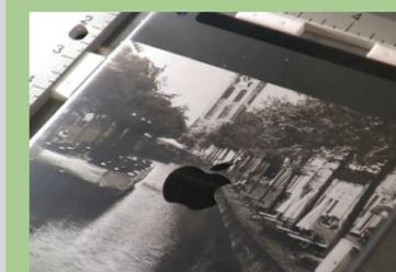
**Tip:** To ensure a flawless alignment, send a vector outline of the Apple logo to the system. Run the job with the door ajar and utilize the Red Dot Pointer. This will allow you to visualize your alignment without making a mark. Make adjustments if necessary.
