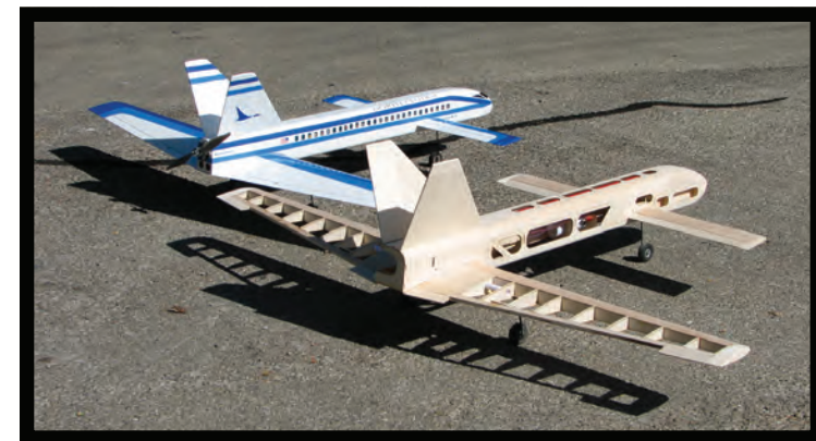
Working radio controlled model plane cut using a laser.
