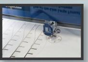
3) Place a sheet of cardboard in the laser and, utilizing the Color Mapping feature and the suggested speed and power settings above, cut 10 pins.
