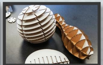
4) Start by inserting the numbered horizontal pieces into one vertical piece in numerical order. Finish by assembling the remaining vertical pieces and glue if desired. You can also increase rigidity and value by experimenting with different 1/8 material such as plywood or acrylics!
