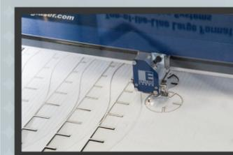
3) Place a sheet of cardboard in the laser and, utilizing the Color Mapping feature and the suggested speed and power settings above, cut 10 pins.
