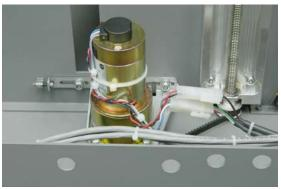
Use a long nut driver to reach the nuts from the side of the machine
