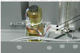
4. Disconnect the white ribbon cable connected to the control board.
