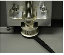
6. Install the belt by following the diagram below. It is easiest to put the belt on the left drive pulley then loop the belt around the right drive pulley.
