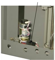
h. Reconnect the white ribbon cable to the control board.
