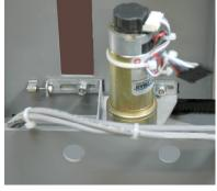
d. Tighten the hexagonal tensioning screw until the edge of the sharpie mark is at the edge of the fixed nut. Getting the precise placement of the sharpie mark is very important. The mark should be in the exact same spot as it was before the screw was taken out.
