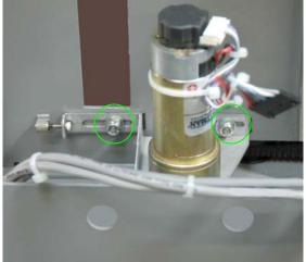
Use a long nut driver to reach the nuts from the side of the machine
