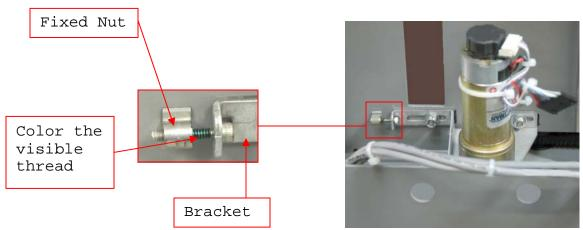
d. With a long 5/16 nut driver, unscrew the two nuts on the motor bracket.
