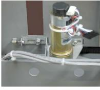
d. Tighten the hexagonal tensioning screw until the edge of the sharpie mark is at the edge of the fixed nut. Getting the precise placement of the sharpie mark is very important. The mark should be in the exact same spot as it was before the screw was taken out.
