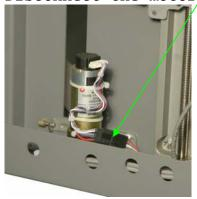
b. Disconnect the white ribbon cable connected to
