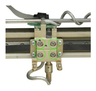
9. Screw in the two 3/32 hex screws to attach the lens.
