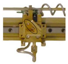
b. Unscrew the four 3/32 hex screws on the lens carriage.
