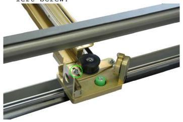
4. Remove the lens assembly from the bearing bracket a. Unscrew the two 3/32 hex screws holding the lens.
