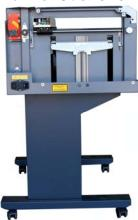
2. Remove the cover off the X-beam.
