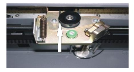
5. Remove the four Philips screws that fix belt to each side of the laser head and leave belt in place.
