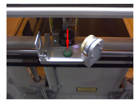
6. By lifting up on both sides of the I-beam, you will free it from the brackets that it sits in. At this point, place the right side of the I beam to the back and bring the left side to the front of the machine. You will be able to slide the I-beam to the right until the left side of the I-beam clears the chassis wall. Now, lift the left side of the I-beam up so the X motor on the right side clears the chassis wall and the I-beam can now be fully removed from the machine.
