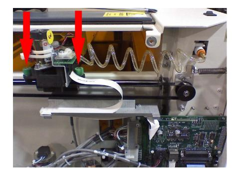
5. Now, loosen the screw with the green casing on the left side of the I-beam using the Phillips head screwdriver.
