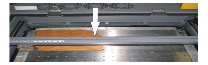
4. Looking at the left side of the I-Beam loosen the Philips screw that sits between the black belt pulley and the spring and push bracket to extend spring to loosen belt tension. View picture 2.
