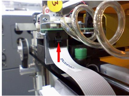
4. Using the Phillips head screwdriver, loosen the 2 screws with the green casing on the I-beam. One is located just to the right and rear of where the white ribbon cable connects and the other is located on the front side of the I-beam, just next to the X motor.
