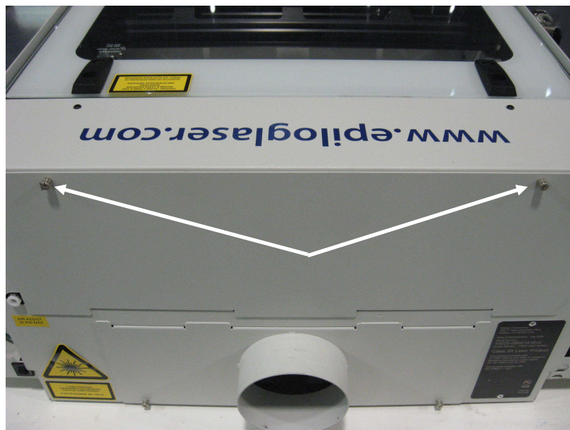
Picture 1 Rear panel screws
