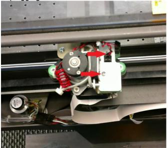
3. Remove the 2 nuts holding the PCB in place and remove it.
