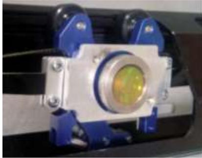
Flip the lens carriage to its normal orientation and pull on the spring loaded wheel and place the carriage back into its track in the gantry.
