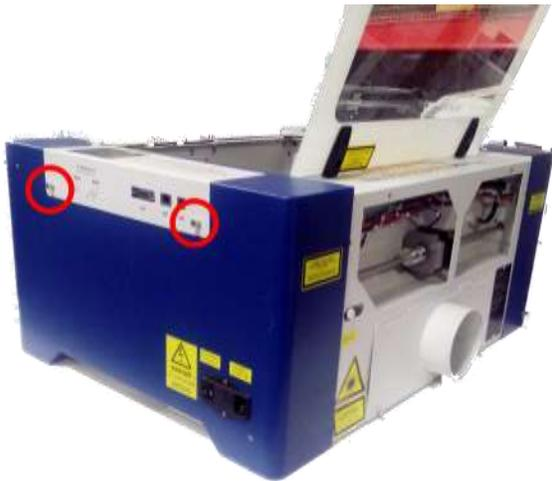
The Captive screws will not come away from the control module. Pull on the Two Captive screws until the Control Module disconnects and slides out from the Control Module Bay. Place the Control Module safely aside.
