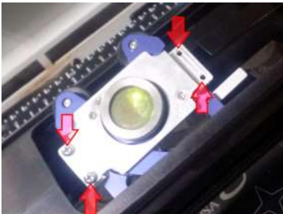
Pull on one end of the belt to free it from the engraver. Do not discard the old belt at this time. Remove the Lens Carriage from the engraver and set it, along with the screws and clamping plates in a safe place for reassembly later. Do not allow the Carriage to rest on the Lens.
