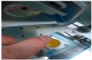
Remember the way the O-ring and lens go. They need to go back exactly the way you removed it. The O-ring should be on top of the lens.
