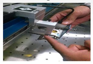
Next, screw the thumb screws back tight on the lens cover. With the M2 Camera, make sure to plug the camera cable back in.
