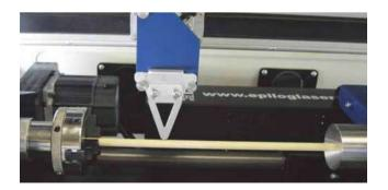
3-Jaw Chuck Rotary Attachment
