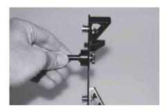
Slide the spindle into the chuck. Make sure the spindle is fully inserted into the chuck, then secure it using the chuck tightening pins.
