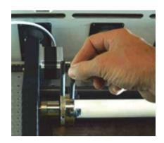
Cylinders can be held from the outside diameter or the inside diameter.
