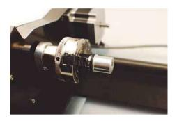
Some parts do not need the idle-side centering fixture for support and can be held using only the 3-Jaw Chuck.
