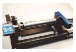
This photo shows a typical example of a larger part that requires a fixture plate on both the left and the right sides. Notice that the left side fixture plate is held in place with the 3-Jaw Chuck.
