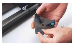
This photo shows the small idle-side plate fixture. The small plate fixture can accommodate sizes up to 1" in diameter.
