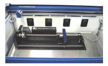
Rotary Attachment until the system is rebooted and you could damage the electronics if the rotary is installed while the laser system is powered on.
