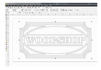
When vector cutting, we always suggest that you use the Vector Cutting Table or Pin Table to protect the back of your material as well as your table from laser marking.
