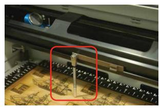
focus anywhere along the X-axis of the table. The focus spring will swing freely when released from its holder.
