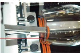
Many glasses, like this one, do not require the use of the clamp. The clamp is used mostly for hard to rotate cylinders or very lightweight objects that need more than just gravity to hold them in place.
