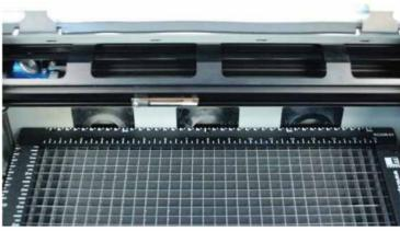
If the Vector Grid is not level, move it further back toward the back wall, then move it around again until the locating pins click into position.
