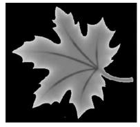
In this sample, the black background would be engraved away. Using this technique, the leaf stands up away from the background, with the edges of the leaf being the highest points and the stems being engraved the deepest.
