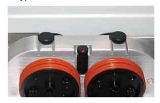
If your Red Dot Pointer is not at this location, you will need to adjust the X- and Y-axis settings to establish the correct Rotary Attachment Home Position. There is an adjustable numerical setting for both the X- and Y-axes that allow you to adjust your Red Dot Pointer so it is calibrated to the edge of the bumper. To change the rotary home settings, follow the instructions below:
