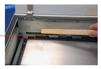
Periodically clean the exhaust plenum at the back of the laser. To access the plenum, remove the two small screws to the left and right of the exhaust port.
