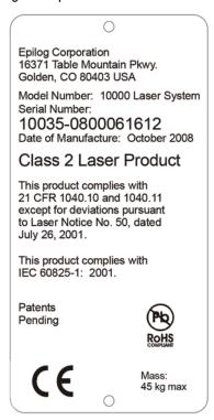
2. **Laser Warning Label:** This label is located on the rear of the machine's cabinet.
