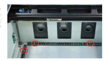
There are three mating pins on the bottom side of the vector grid that fit into the slots in the ruler.
