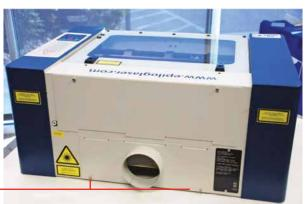
Clean the plenum with a flexible plastic or wire brush that can access the inside of the port. Inspect and clean your exhaust fan and duct work connected to the port.
