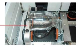
Use the scissor jack to raise the right side of the cylinder so that the engraving surface is horizontal. The photos below show the same flashlight at a severe angle to horizontal. If your cylinder is not horizontal to the X-beam, the laser will lose focus as the carriage head moves across the flashlight. This causes the engraving quality on the right hand side to suffer dramatically.
