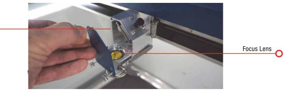
In addition to the focus lens and the mirror directly above it, there is a mirror located on the left side of the X-beam. This mirror is very well protected and should not need regular cleaning. It can be accessed with a cotton swab if it does need cleaning.
