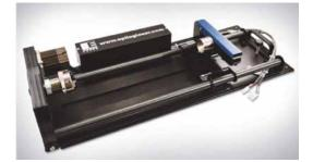
This photo shows the 3-Jaw Chuck style Rotary Attachment with the large fixture plates installed.
