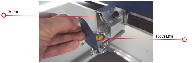
To clean the optics, use a high-quality cotton swab moistened with the optics cleaner supplied in the accessory kit. Please read the label on the bottle carefully.
