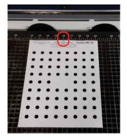
5. After properly placing the calibration form, click the **Proceed** key.
