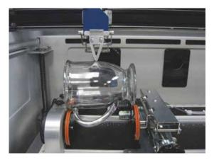
When you are finished focusing press the **Reset** key on the Control Panel. Pressing Reset will send the lens carriage back to its standard Home Position at the front of the black bumper. You are now ready to start the job.
