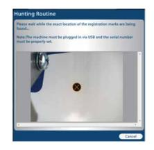
After locating the second mark, the carriage will stop moving while it is directly over the second mark. At this point, the vector files is transferred to the Fusion and the Fusion is ready to start cutting.
