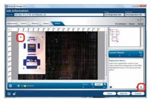
10. After clicking the second registration mark the video feed will show an overlay of vector lines to be cut. Insure the lines are in the correct location and orientation. If they are, you are ready to print to the Fusion.
