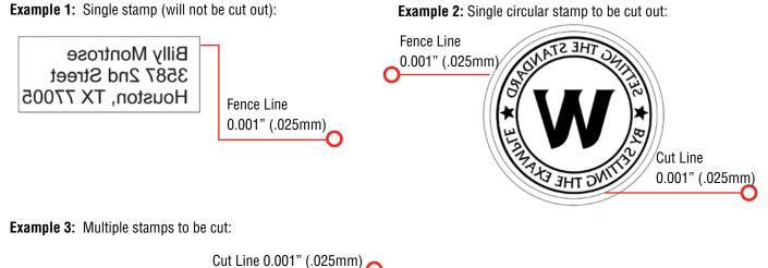
Cut Line 0.001" (.025mm) Cut Line 0.001" (.025mm) Cut Line 0.001" (.025mm) One fence to surround all stamps.
