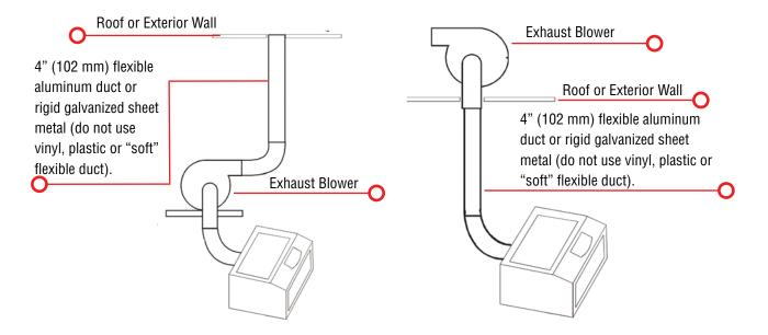
The drawings above show the typical exhaust setup. The left drawing shows the exhaust near the machine and the right drawing shows the exhaust fan on the roof. Where the exhaust fan is placed is a choice of personal preference. Some users like the exhaust fan outside because of noise considerations.
