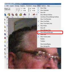
9. **Crop the Photo:** If you do not want to engrave the entire photo, double click on the photo to open the bitmap tools at the top of the page. Select the Rectangle or Ellipse tool to frame the area you want to crop. With the proper area framed, press the Crop key to finalize the crop.
