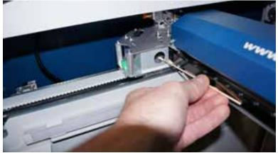
The photos below shows how to clean the focus lens. Remove the lens carriage from the machine to clean both the top and bottom of this lens.
