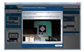
5. When finished, the calibration video feed will disappear and the Calibration Complete window will appear. **Press OK**.
