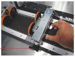
Rotate the knob to lift or lower the scissor jack.
