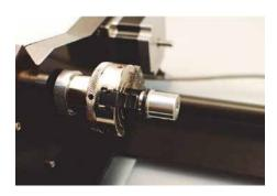
Some parts do not need the idle-side centering fixture for support and can be held using only the 3-Jaw Chuck.
