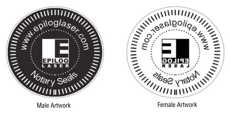
The male image should be produced without the use of outlines around the text or graphics. Add a .007 to .010 inch (0.178 mm to 0.254 mm) outline to the text and graphics of the female die. This outline creates a large enough void between the male and female dies to emboss paper without tearing.
