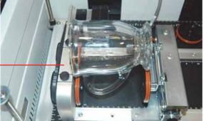
Use the scissor jack to raise the right side of the cylinder so that the engraving/cutting surface is horizontal. The photos below show the same flashlight at a severe angle to horizontal. If your cylinder is not horizontal to the X-beam the laser will lose focus as the carriage head moves across the flashlight. This causes the engraving quality on the right hand side to suffer dramatically.
