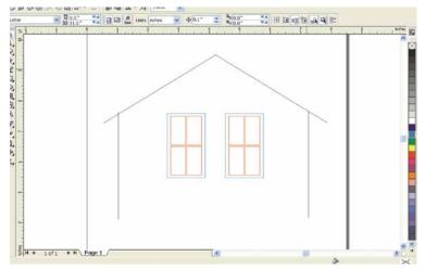
3. In our example we want to mark the green window frames first, so green must be the first color at the top of the list. Normally the color green is the second color down in the list. In order to move it we just select it and press the **Up key** to move it up one position. We now have green at the top and red is the second color down. This is the order that the colors will be processed.
