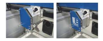
2. Install the 3" lens. Notice that the 3" lens does not include the Crash Bar or Air Assist tube.
