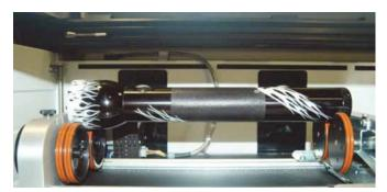
Correct Setup: The flashlight is horizontal to the X-beam
