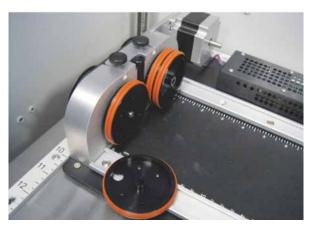
There are two small thumbscrews that attach each front drive wheel to the back drive wheel. Loosen the two small thumbscrews on each wheel to remove the front wheel.
