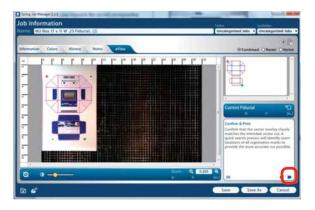
11. **Hunting Routine:** The laser carriage will start moving to find the first registration mark and precisely locate its exact location on the laser bed. The same process is followed to precisely locate the second mark.
