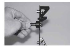
Slide the spindle into the chuck. Make sure the spindle is fully inserted into the chuck, then secure it using the chuck tightening pins.
