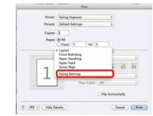
Set your laser Settings. We've set our Job Type to Combined because we'll be both engraving and cutting in this job. For Raster Settings, we've used 50% speed, 100% power. For Vector Settings, we've used 30% speed, 70% power. Finally, our resolution has been set to 600 DPI.
