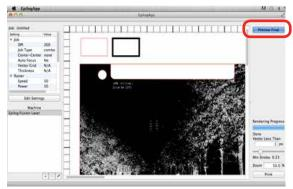
In this example, you can see there are red vector lines that will vector. There are red lines that make up the iPad Air template, used for alignment, and another red box above the photograph.
