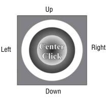
You can adjust the default laser power being used in Laser On mode from the Settings menu. Highlight Settings, then use the Joystick to scroll down to Jog Laser PWR. Center click the Joystick and then tilt the Joystick Up or Down to change the value. Press the Go key to activate the change. Go back to Jog mode to use Laser On.
