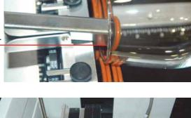
Many glasses, like this one, do not require the use of the clamp. The clamp is used mostly for hard to rotate cylinders or very lightweight objects that need more than just gravity to hold them in place.
