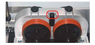
To establish the Rotary Home setting at the front of the black bumper we will use the Red Dot Pointer to show us where our Home Position is and then how far we need to adjust our settings. Once you have set and saved the X and Y Rotary Home Position you should not have to set it again.
