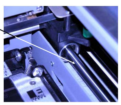
Clean the length of the left side Y-axis rail using a soft cotton cloth. Lubrication is not required.
