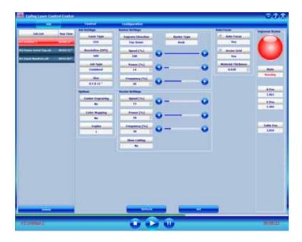
At the bottom of the ECC you can see a visual indicator in green that shows the progress of the job. As you can see, this job is about 2/3rds complete and has been running for 23 seconds.
