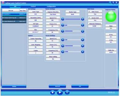
The image below shows that Job #3 has now been completed because there is no asterisk in the Run Time section.
