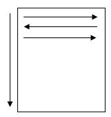
Top-down engraving starts from the top and works its way down.
