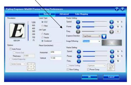
This feature applies to Raster engraving only and allows you to engrave your project either from the top down, or the bottom up. This is very helpful for some materials like plastic or rubber stamps. In standard top-down engraving there can be a large amount of engraving debris generated. As the debris moves towards the exhaust plenum, some of it collects in the area that has just been engraved. Bottom-Up engraving prevents the debris from collecting in the freshly engraved spaces.
