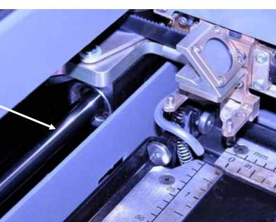
After cleaning the rails and bearings, clean off the table and the rest of the inside of the machine. Spending just a few minutes a week will pay off in the long run with better quality and performance.
