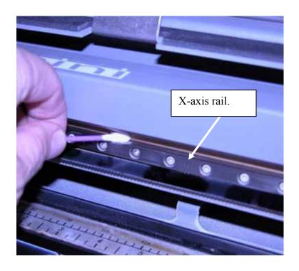
After cleaning the rail, place about an inch long bead of Epilog supplied grease into the top and bottom grooves of the X-axis rail. The following photo shows where to grease the bottom groove of the rail.
