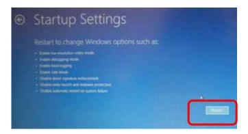
9. Press either the F7 key or the number 7 key from your computer keyboard. This selection disables the Driver Signature Enforcement which will then allow you to install a printer driver.
