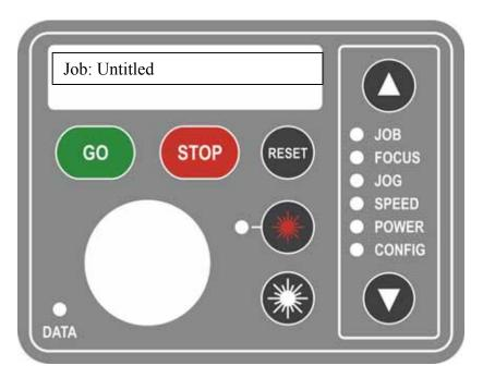
Place your work piece in the upper left corner of the engraving table, close the door and then press the Go key to start the job.
