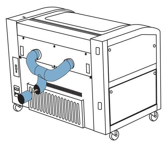
There are two 4" (100 mm) ports attached to the back of the laser system. Attach your ducting to the machine as shown above.
