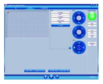
You can use the buttons at the bottom of the screen to set a temporary Home position or to send the carriage back to its standard rest position.
