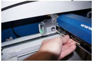
The photos below shows how to clean the focus lens. Remove the lens carraige from the machine to clean both the top and bottom of this lens.
