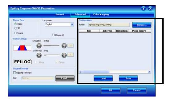
The "Configurations" feature is a comprehensive data management tool that is used to save all of your Dashboard settings for individual jobs. Saving the Dashboard settings as a database file allows you to retrieve the job parameters at a later time. This saves you the trouble of trying to remember what speed and power and other settings you used on a job you did three months ago. All of your settings can all be stored as a permanent record.
