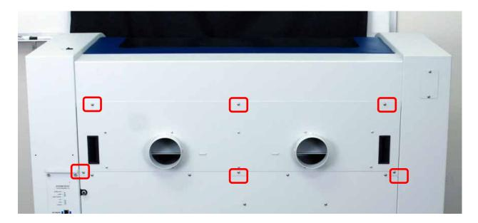
The photos below the plenum partially removed and the back of the machine with the plenum fully removed.
