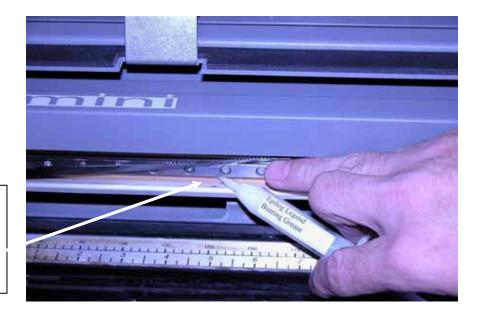
Place a bead of grease along the bottom groove of the X-axis rail.
