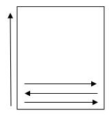
Bottom-Up engraving starts from the bottom and works its way up.
