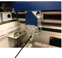
Place the manual focus gauge on the carriage and place the object to be cut or engraved in the upper-left corner of the machine. Use the arrow keys on the control panel to highlight the light next to the word *Focus*. You can now move the *Joystick* up or down to move the table appropriately until your material just touches the bottom of the gauge. The speed at which the table rises or lowers can be controlled by applying varying pressure upwards or downwards on the
