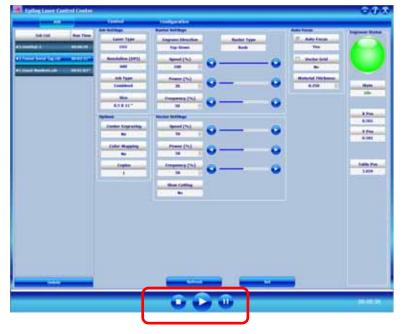
The Job tab allows you to run the laser from this one page once a job has been printed to the laser.
