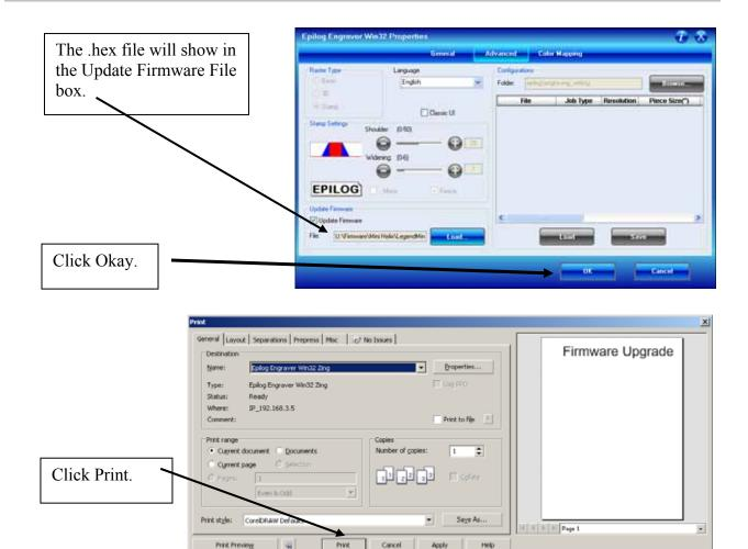
At this point, the .hex file will begin transfering to your laser. The laser knows that it is being upgraded and the graphic that you created will not print, nor will it show up as a Job. Instead, you will see the a message on the LCD panel on the laser. When you are asked to reboot the process is complete.
