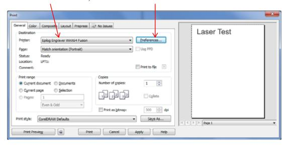
Set your laser parameters for the test job and then press Okay. For this test job the laser parameters are not overly important. We are just making sure the computer and laser are talking to each other and that a job can be sent and will start running.
