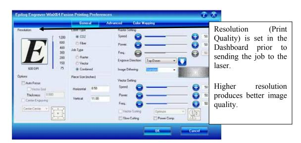
Speed and Power settings are dependent on resolution setting. For example, there is greater overlap of each raster line at 600 DPI than there is at 300 DPI. The additional overlap at 600 DPI has the effect of lasering over more of each line twice. This means that on material like wood, you will notice a greater depth of engraving at 600 DPI than you will at 300 DPI if you use the same Speed and Power settings.
