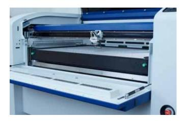
The struts can be disconnected if you wish to open the door more than its standard 90 degree opening. Remove the left and right thumb screws to allow the door to open the full 180 degrees.
