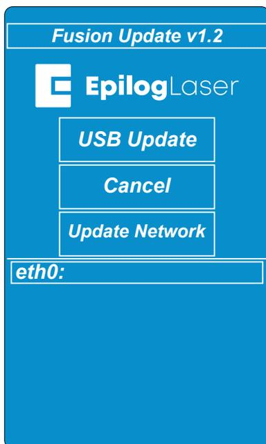
3. Open your web browser and in the search bar, type "**http://**" followed by the IP address currently displayed on the Fusion Edge's screen next to "eth0:". After the IP address, add "**:8080**" and hit "**Enter**".
