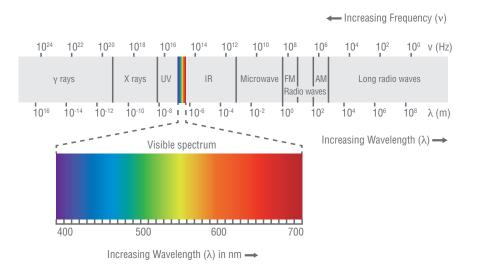
For purposes of understanding lasers, we generally think of light as electromagnetic radiation having wavelengths ranging from around 10 nm (the bottom of the ultraviolet, or UV, portion of the spectrum) up to about 1,000,000 nm (or 1 mm, the top of the infrared, or IR portion).
