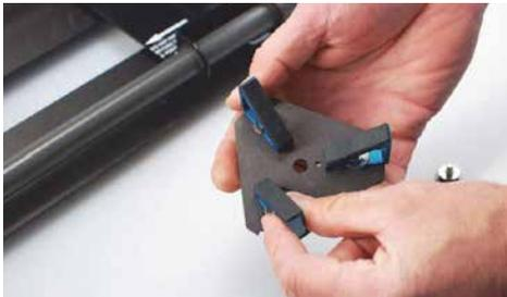
This photo shows the small idle-side plate fixture. The small plate fixture can accommodate sizes up to 1" in diameter.
