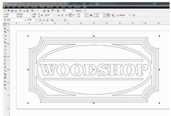
When vector cutting, we always suggest that you use the Vector Cutting Table or Pin Table to protect the back of your material as well as your table from laser marking.
