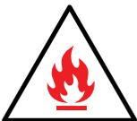
This icon indicates the potential for fire damage when operating the laser.
