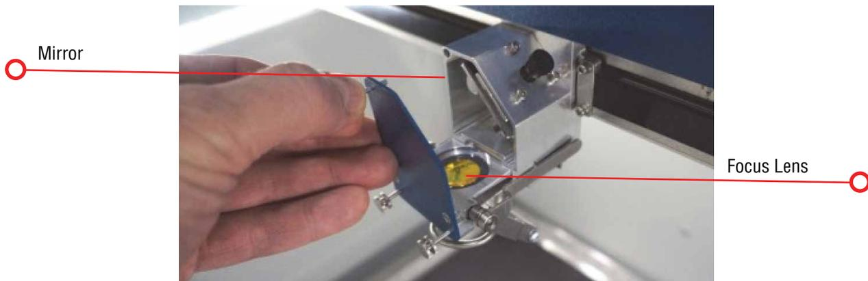
To clean the optics, use a high-quality cotton swab moistened with the optics cleaner supplied in the accessory kit. Please read the label on the bottle carefully.
