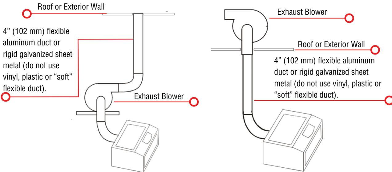
The drawings above show the typical exhaust setup. The left drawing shows the exhaust near the machine and the right drawing shows the exhaust fan on the roof. Where the exhaust fan is placed is a choice of personal preference. Some users like the exhaust fan outside because of noise considerations.
