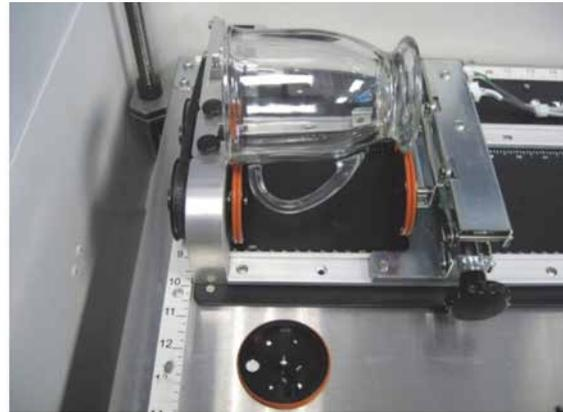
This photo shows a mug with a handle positioned on the Rotary Attachment with the removable portion of the drive wheel shown in the foreground.
