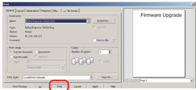
At this point, the **.hex** file will begin transferring to your laser. The laser knows that it is being upgraded and the graphic that you created will not print, nor will it show up as a Job. Instead, the cursor keys will light up. When the upgrade is complete, the display will read **Reboot!**
