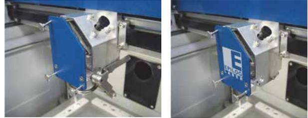
2. Install the 3” lens. Notice that the 3” lens does not include the Crash Bar or Air Assist tube.
