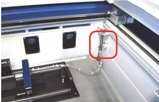
5. Once the Rotary Attachment is plugged in you can power on the Fusion.
