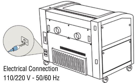
The Fusion 120 watt laser system requires 208/220/240 volt electrical power. This system will not operate on 120 volt power. The Fusion 120 watt power cord comes with a male plug type NEMA L6-15R (which is a Hubble HBL4570C equivalent).
