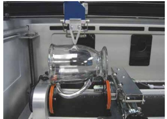
When you are finished focusing press the **Reset** key on the Control Panel. Pressing Reset will send the lens carriage back to its standard Home Position at the front of the black bumper. You are now ready to start the job.
