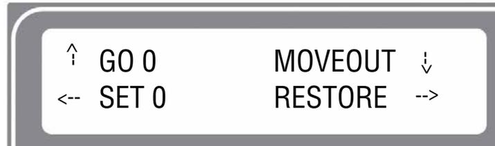
The sub-menu shows that a down tilt of the Joystick will “Moveout” the X-beam. The Moveout command will move the lens carriage back from Home so that the focus gauge is centered over the cylinder.
